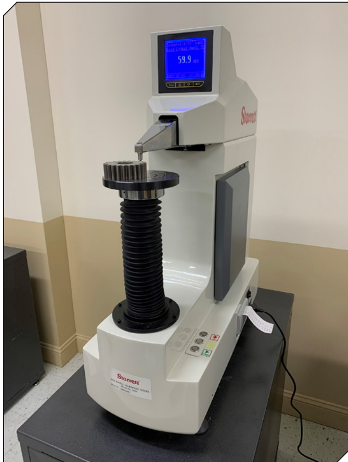
Starrett digital Rockwell/Superficial Rockwell Benchtop Hardness Testers feature fully automated load/unload procedures, and are capable of providing highly accurate readings.
