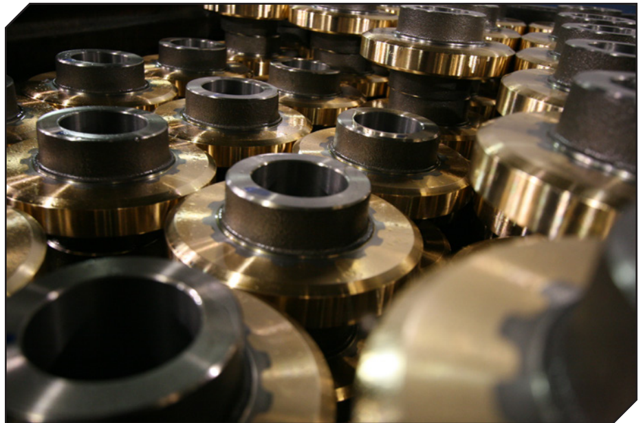
The continuous cast process allows for part-specific casting, where simple features can be continuous cast into the raw material, thus providing a near-net shape.
