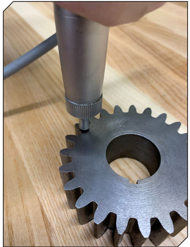
Starrett 3821 Ultrasonic Portable Hardness Tester will test gear teeth nondestructively and can read in just about any scale at about two seconds.
